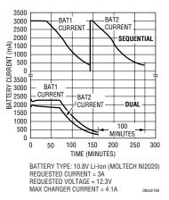
Figure 2. Dual Battery vs Sequential Battery Charge Time
