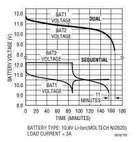
Figure 3. Dual Battery vs Sequential Battery Discharge Time
