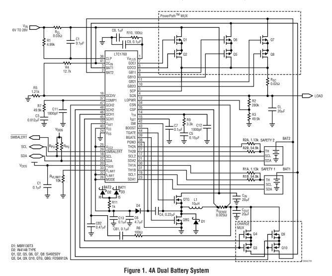
ducing any audible noise. The high 300kHz switching frequency allows the use of small low cost  $10\mu$ H inductors.
